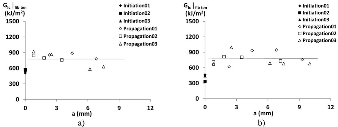
**Figure 7.** R-curve obtained from a) Area method and b) Compliance calibration
