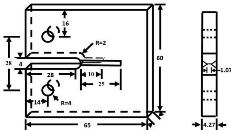
**Figure 1.** Dimensions of GCT specimen (all dimensions are in mm)
