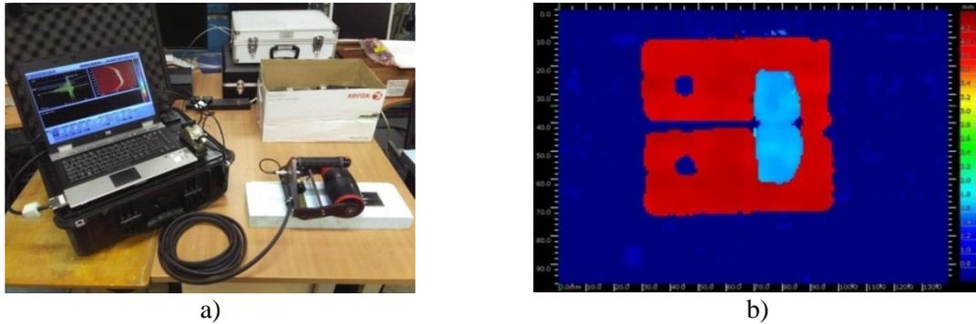
**Figure 5.** a) Ultrasonic scan system b) measured debonding area
