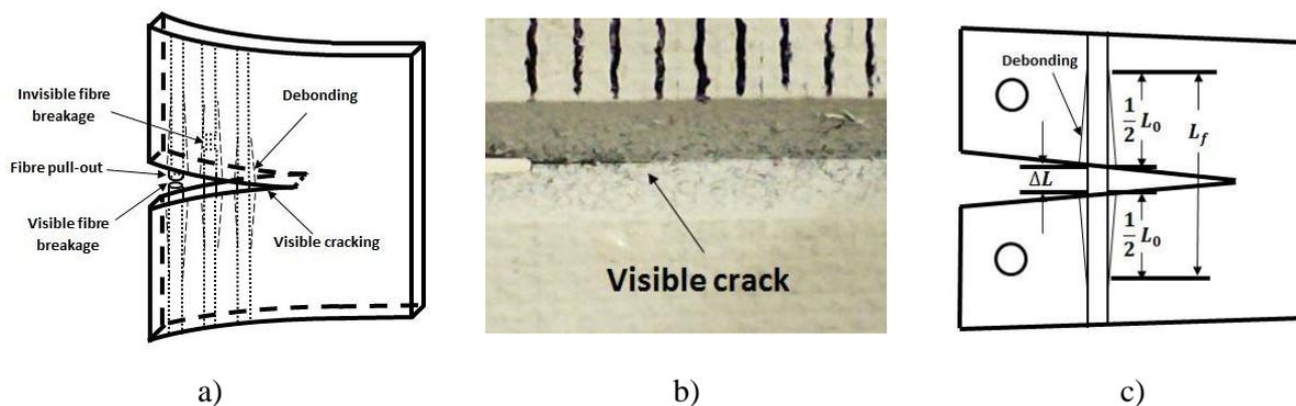
**Figure 4.** a) high risk regions and b) visible cracking c) definition of localized linear strain
