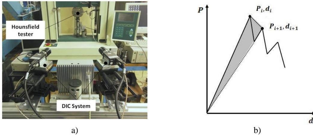
**Figure 3.** Photographs of a) experiment set-up b) The definition of the area method
