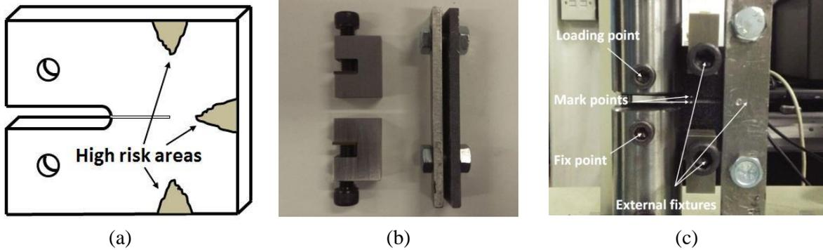
**Figure 2.** a) Susceptible regions b) external fixtures and c) assembly of specimen and fixtures.
