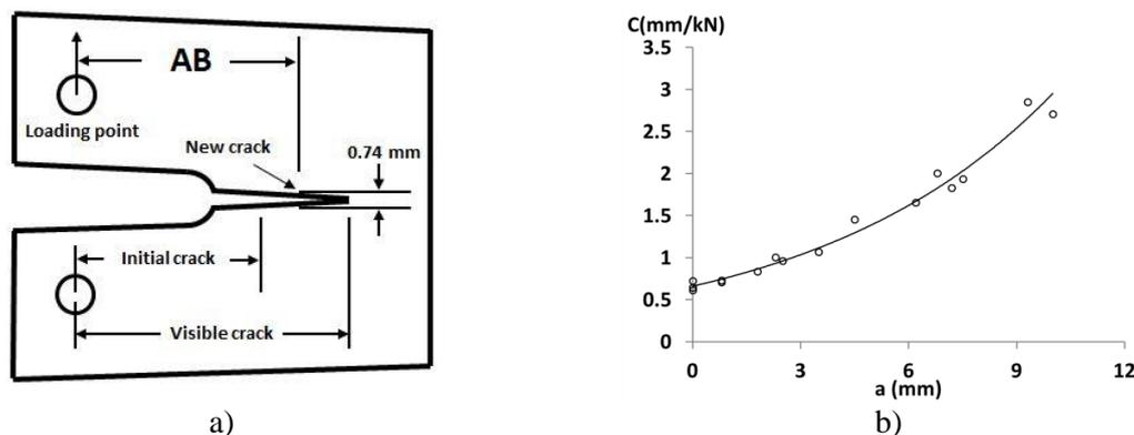
**Figure 6.** a) Determination of crack tip b) Compliance versus crack length
