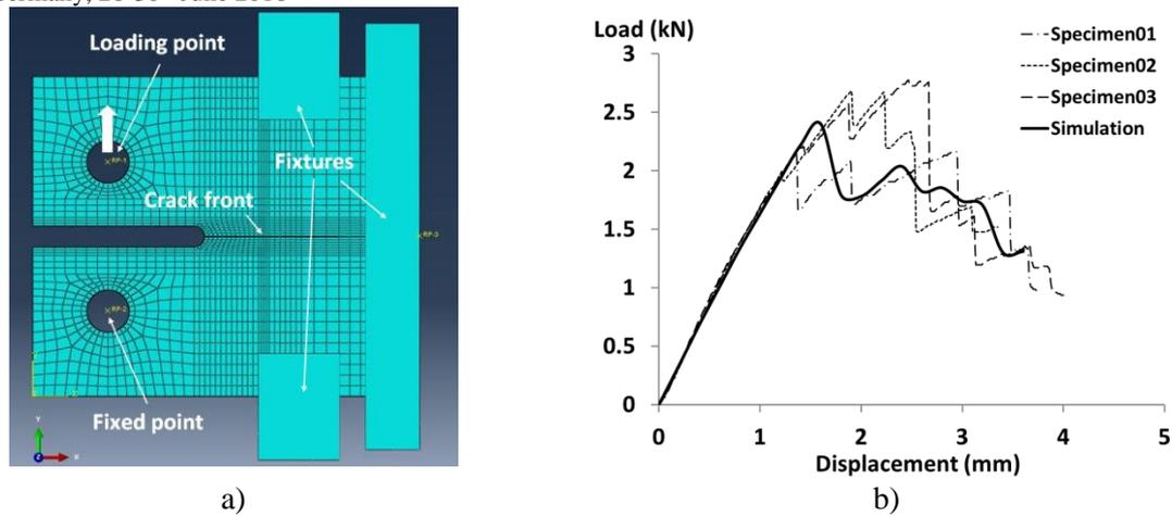
**Figure 8.** a) FE model and b) Load-displacement curves from simulation and experiment
