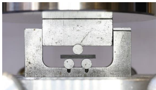
Figure 2. Short beam shear experimental set-up
