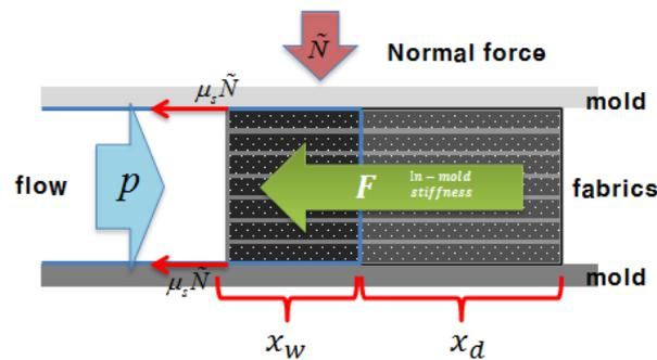
**Figure 1.** Schematic diagram of relating forces during resin impregnation in liquid composite molding
