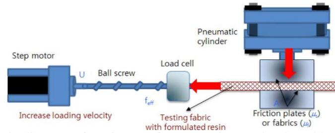
**Figure 2.** Schematic diagram of equipment for measuring coulomb and hydrodynamic friction coefficients
