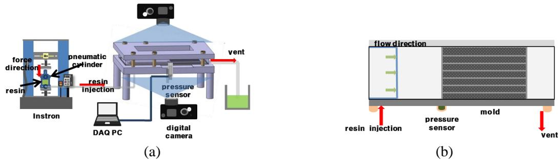
**Figure 4.** Schematic diagram of equipment for measuring flow induced deformation of fiber preform in liquid composite molding. (a) overall equipment, (b) inside of mold
