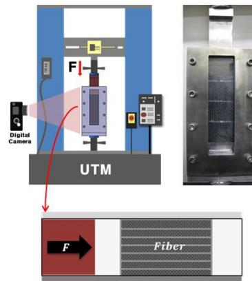
**Figure 3.** Measurement system for in-mold stiffness of fiber preform
