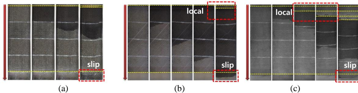
**Figure 5:** Deformation image of fiber preform in various orientation angles. (a) 0°, (b) 45°, (c) 90°
