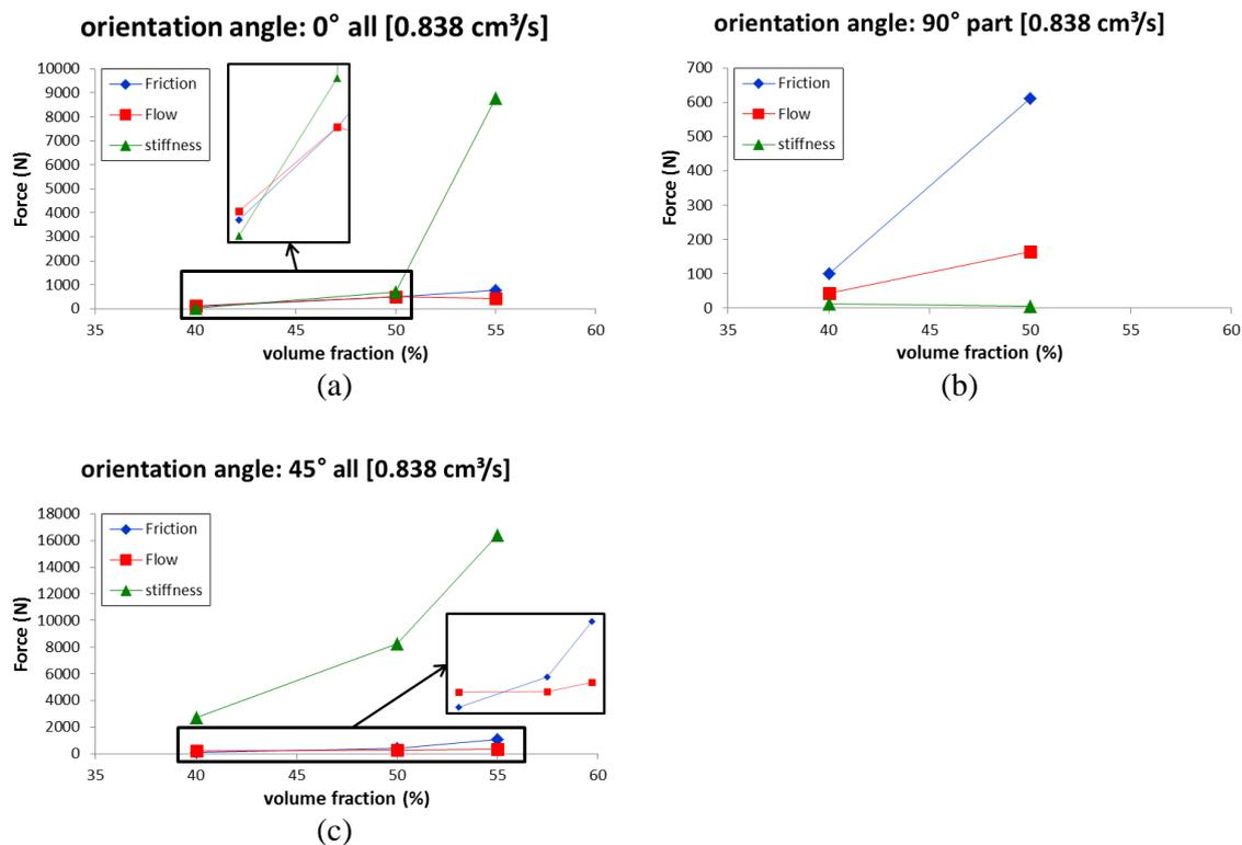
Figure 6: Comparison of the related forces for the various fiber deformations: friction, flow and in-mold stiffness induced force. (a) slip (UD 0°, 0.838 cm<sup>3</sup>/s), (b) wrinkle (UD 90°, 0.083 cm<sup>3</sup>/s), (c) wrinkle (UD 45°, 0.083 cm<sup>3</sup>/s)
