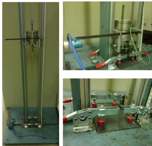
Figure 2: Images of the testing machine used for the performance of the low velocity tests.
