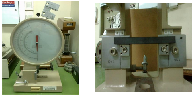
Figure 1: a) Universal testing machine Karl Frank GMBH, b) Presentation of the supported V-notched specimen.
