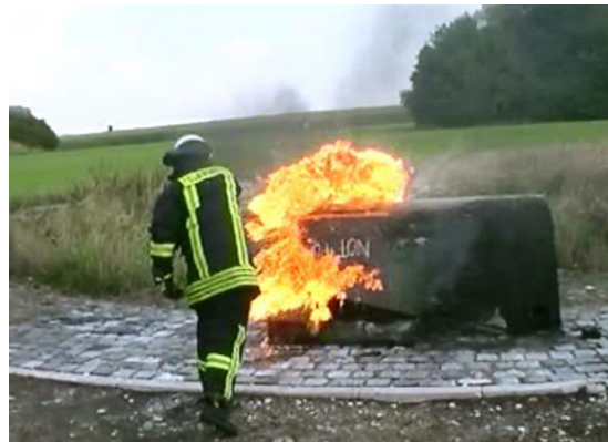
Figure 4. Helicopter CFRP sandwich structure during application of improvised fire accelerant
