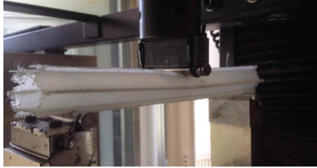
Figure 8 Bending test one hexagonal cavity.
