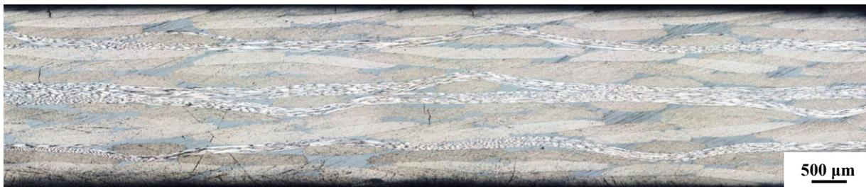
**Figure 4** Representative cross-section from the laminate acquired by optical microscopy [5].
