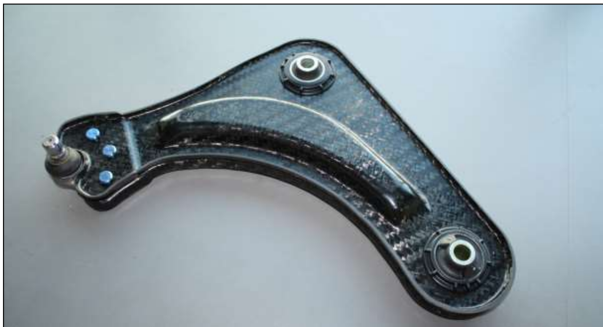
Figure 3. Thermoplastic composite suspension arm made of organosheet plates : fulfilled the mechanical specifications, high volume production was possible but cost too expensive compared to the one of a steel arm. This prototype made by Cetim and Onera in 2012 [1-2] was the starting point of the QSP® concept.
