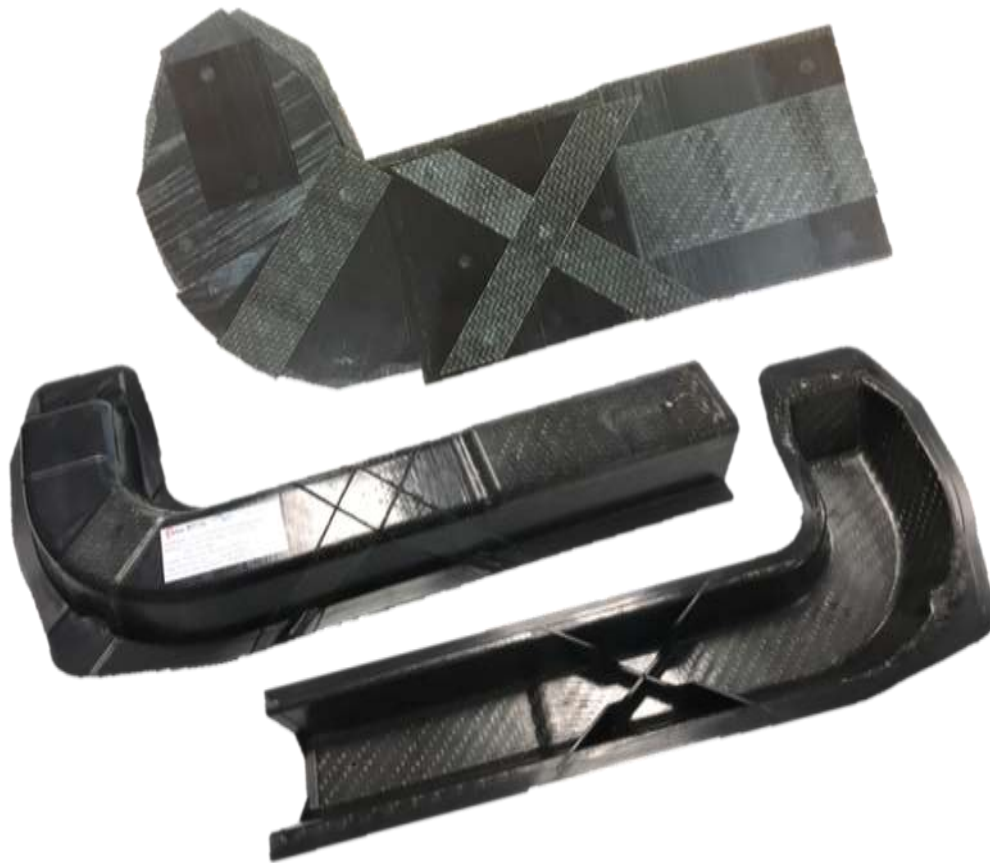
Figure 6. Example of multi-thickness QSP® part made of the netshape blank shown on the upper side of the figure
