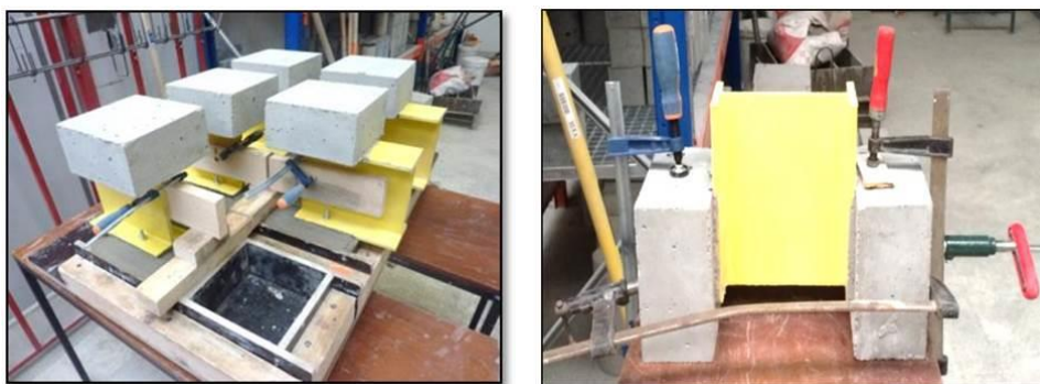
Figure 2. Specimen preparation (left) Casting of bolted specimens (right) Bonding between GFRP and concrete
