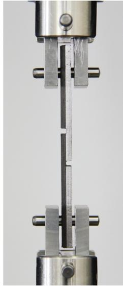
**Figure 3.** A lap shear sample loaded for testing
