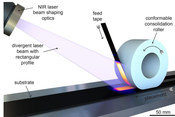
**Figure 1.** A typical laser TP-ATP manufacturing process.
