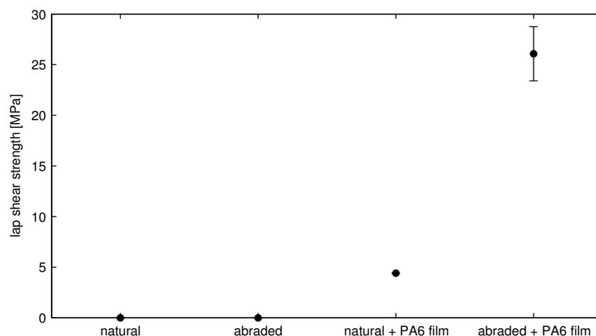
**Figure 4.** The effect of various surface treatments on lap shear strength.
