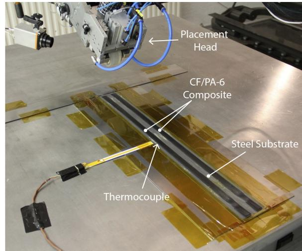
**Figure 2.** Two parallel strips of CF/PA 6 applied to a steel substrate.
