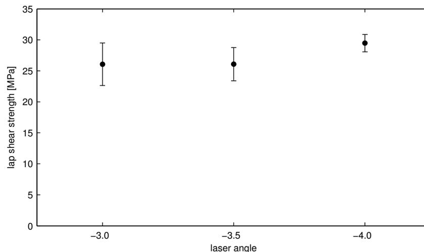
**Figure 5.** Effect of laser angle for grit blasted substrates with a PA 6 film applied
