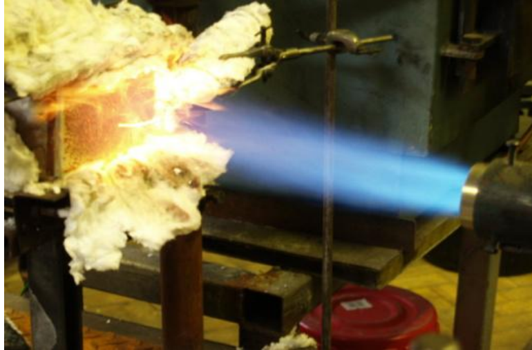
Figure 1. Fire test set up.
