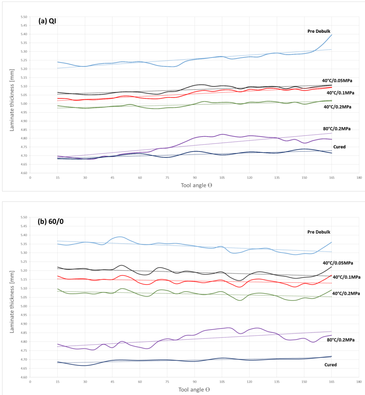
Figure 2 Thickness variation around laminate radius in Fig. 1 at different temperatures and bag pressures \sigma_n for (a) QI and (b) 60/0 laminates
