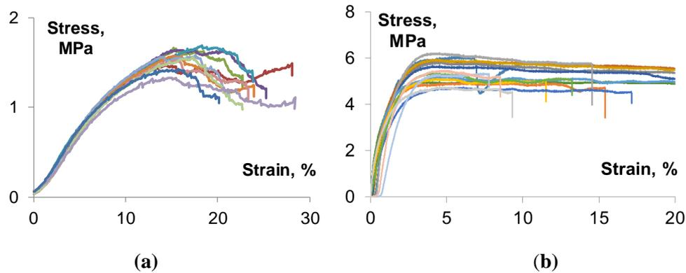
**Figure 2.** Stress – strain curves of: material of microcapsules shell (MF resin), compression (a); pure PVA matrix specimens, tension (b).
