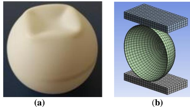
**Figure 4.** Testing and modelling: deformed shape of ping pong ball (a); FE model (b).
