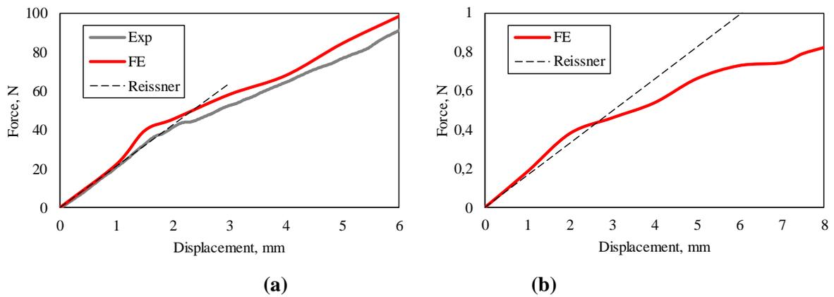
**Figure 5.** Dependences of compression force upon displacement obtained: experimentally, by finite element modelling and theoretical Reissner equation for nitrocellulose ping pong ball (a); by finite element modelling and theoretical Reissner equation for a ball from MF resin (b).
