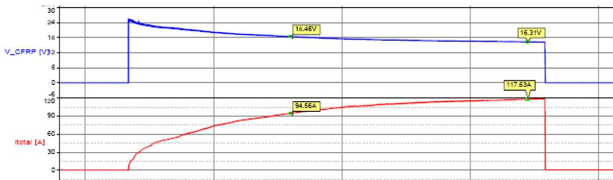
Figure 6. Measurement of the coupon voltage (top) and current (bottom) during degradation.
