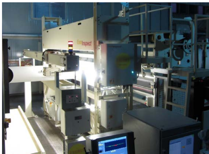
Figure 1. Optical in-line inspection system for quality and process control of composites
