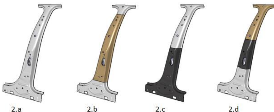
Figure 2.a conventional appearance, 2.b, 2.c, 2.d some possible material distribution of B-Pillar
