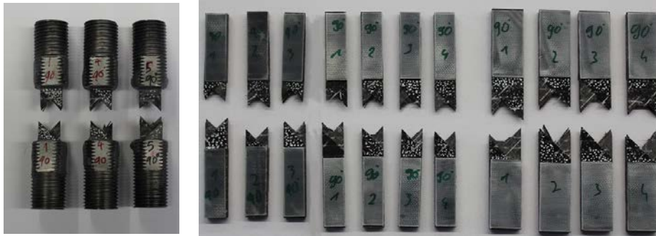
Figure 7. Failure patterns of specimen with end caps (left) and tested in the alternative mounting (right)
