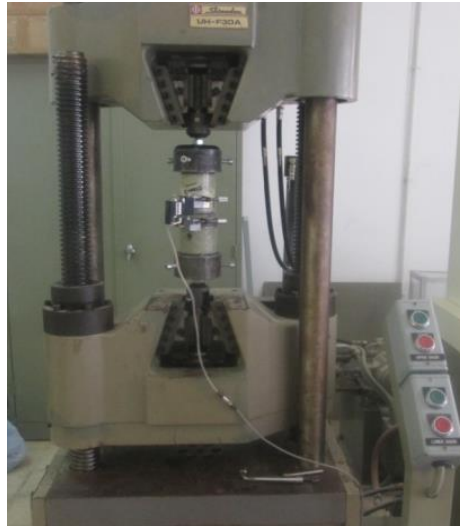
Figure 2. Experimental device developed for joined specimen for tensile test
