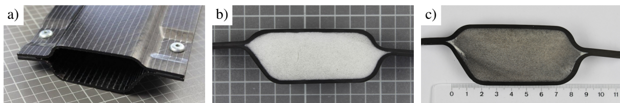
Figure 5. Prototype parts: modular shell construction (a), sandwich part with a milled PMI-E core (b) and sandwich part with a thermoformed PET-E core (c).
