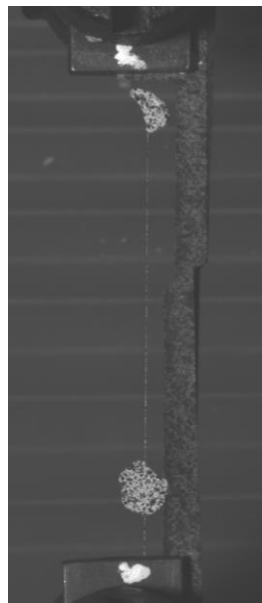
Figure 2. Mounted testing frame containing a single fibre with optical flags attached to it.
