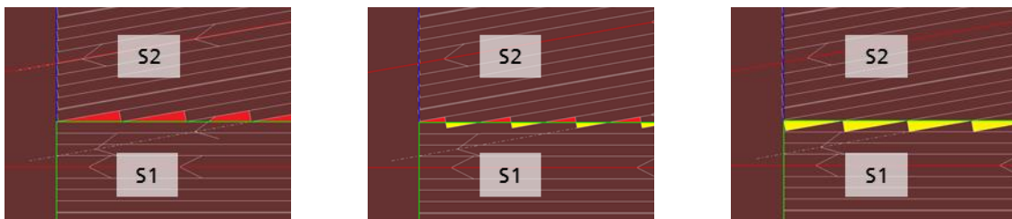
Figure 3. Boundary design by overlap parameter: O_{S2} = 0\% , O_{S2} = 50\% , O_{S2} = 100\%
