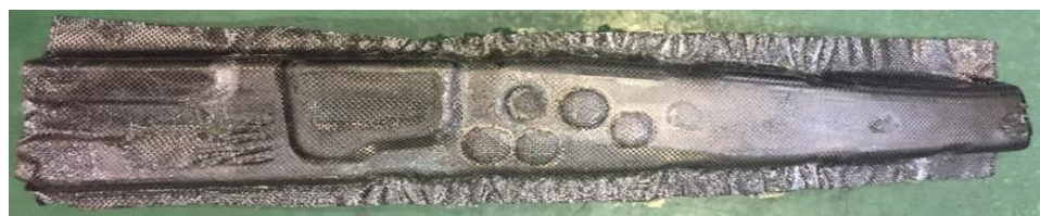
(a) Before piercing and trimming
