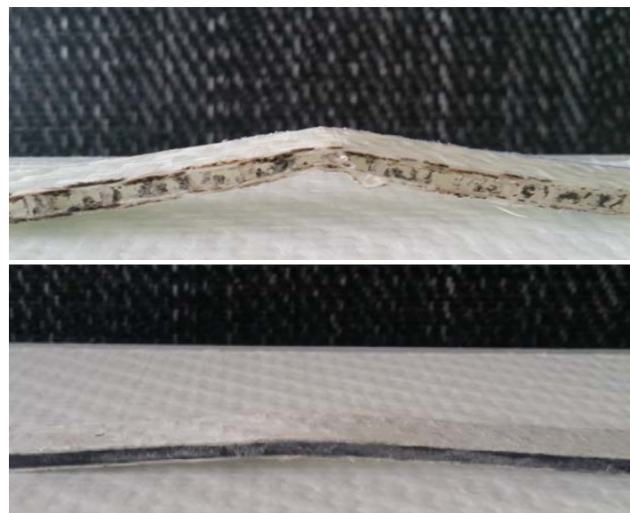
Figure 4. A view of honeycomb and RPP foam sandwich panels after the bending test
