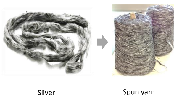
Figure 3. View of sliver and yarn manufactured by the developed method.
