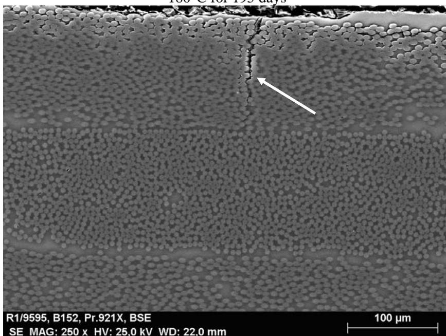
Figure 4: SEM photograph; zooming part of the cross-section of a specimen thermally degraded at 180° for 195 days and loaded in tensile mode with 0.3% strain
