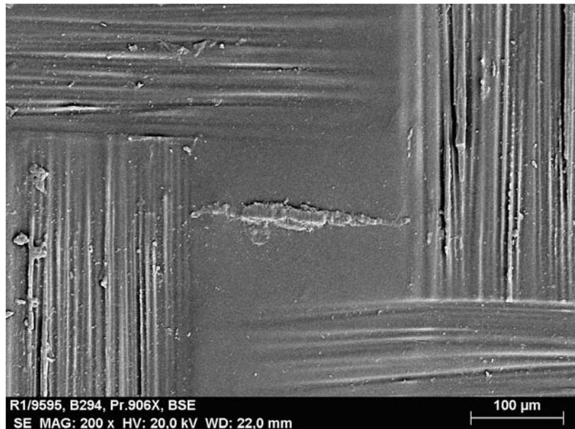
**Figure 1:** SEM photograph; non-thermally degraded surface of a specimen showing no cracks parallel to the outermost ply
