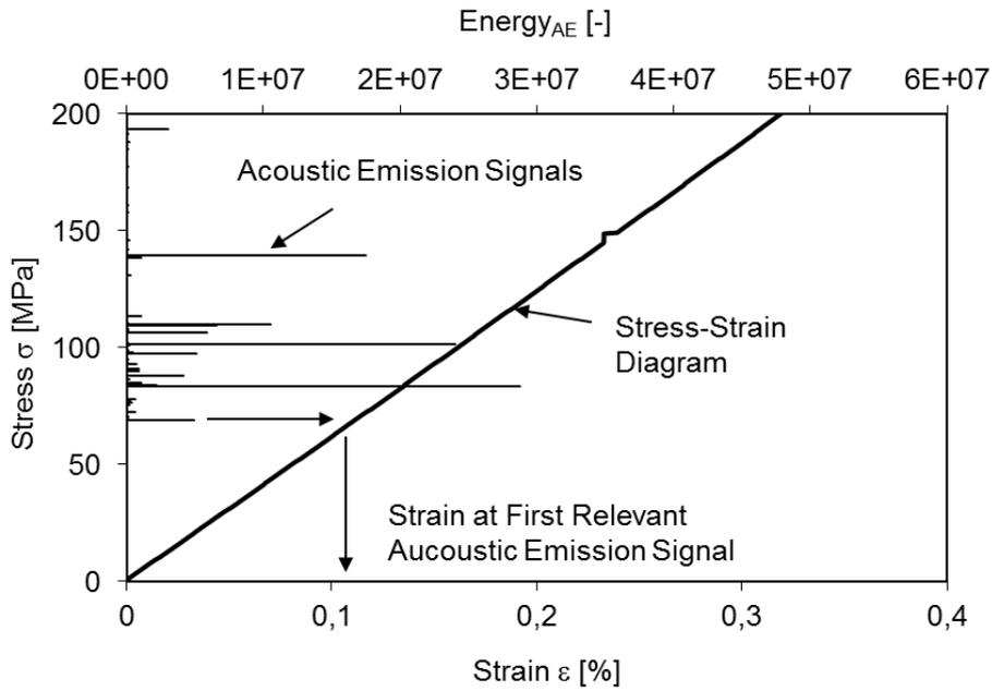
**Figure 6:** Thermally degraded at 200°C for 195 days, stress-strain diagram and acoustic emission signals
