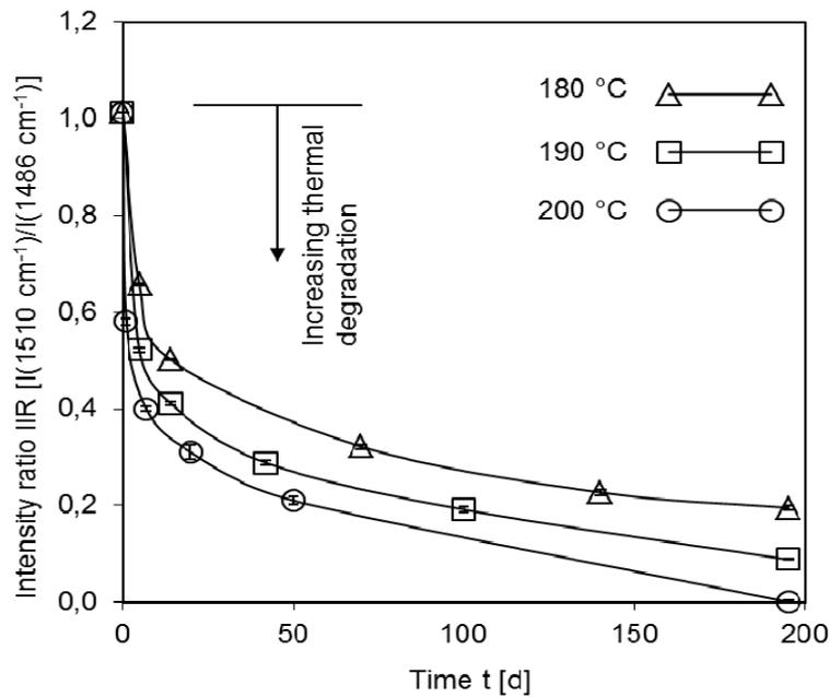
**Figure 7:** Intensity ratio vs. storage time of thermal degradation
