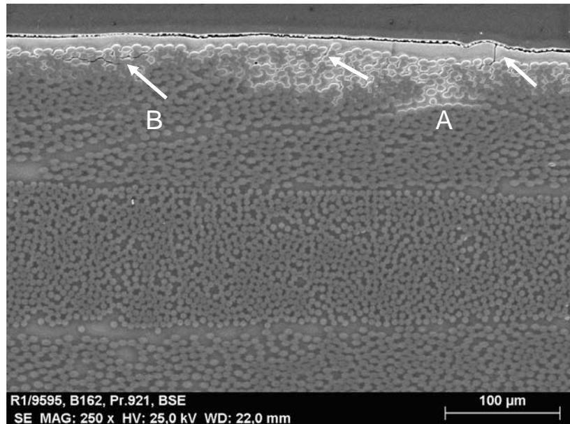
Figure 3: SEM photograph; zooming part of the cross-section of a specimen thermally degraded at 180°C for 195 days
