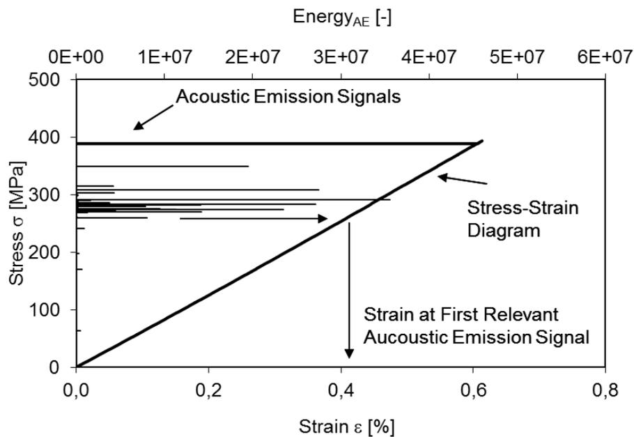
Figure 5: Non-thermally degraded; stress-strain diagram and acoustic emission signals
