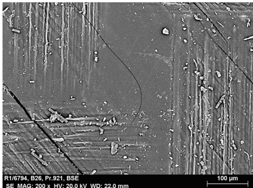
**Figure 2:** SEM photograph; degraded at 180°C for 195 days showing cracks on the outermost ply
