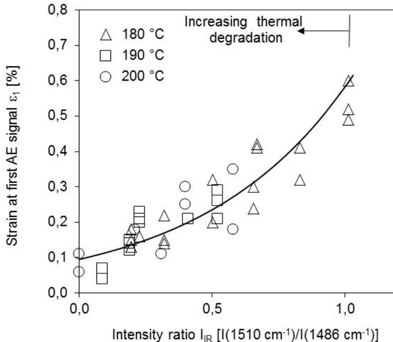
**Figure 8:** Evaluated strain at first significant acoustic emission energy peak at all three aging temperatures vs. thermal degradation characterized by IR intensity ratio
