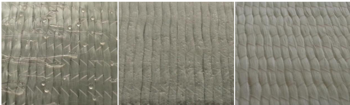
Figure 3. Example of different textures when using different binder application parameters: drop or fiber like texture (left), web like texture (middle), fine silky coating (right)
