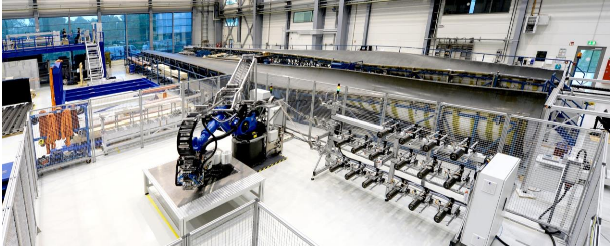
Figure 1. Manufacturing area for wind turbine rotor blades at the ZLP with the DRP unit and a 45 m rotor blade tool.
