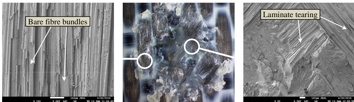
Figure 9. Fracture surface of the spot-welded joint after PT tests (middle). The left and right images show SEM details for the failure modes, indicated by the left and right white circles on the fracture
