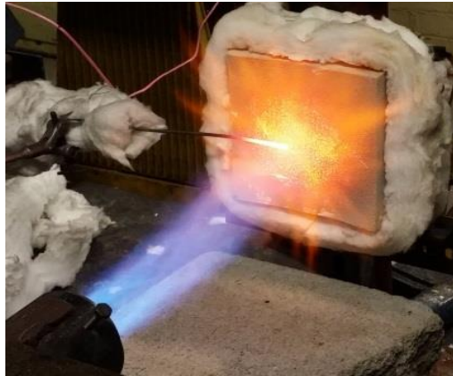
Figure 1: Propane burner test set-up for measurements on composite PFP.
