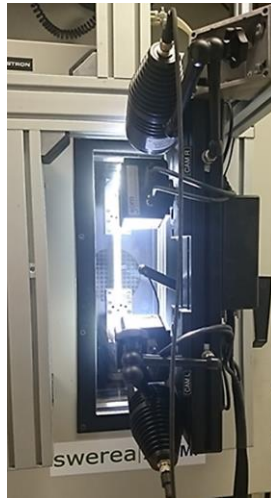
Figure 3. Setup of the GOM Aramis system for for tensile testing at 320°C [11].
