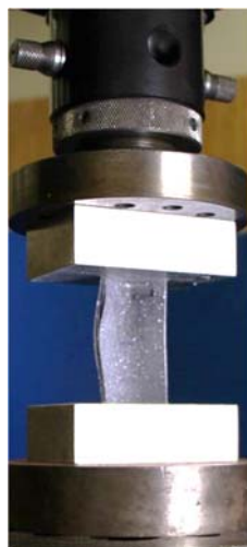
Figure 8. Buckling of corner compression test sample
