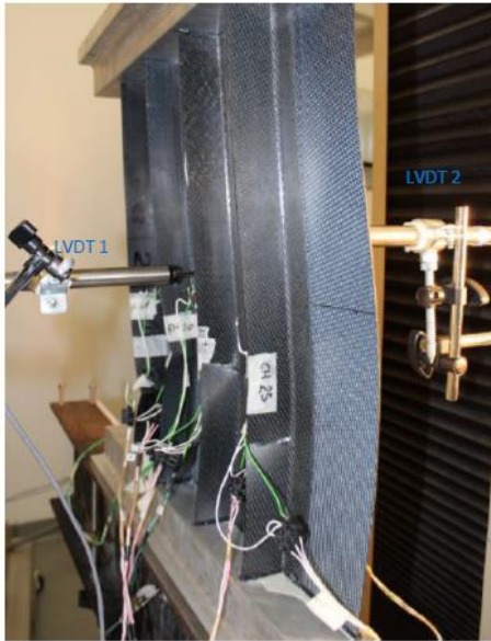
Figure 7: buckling test set-up for the panel
