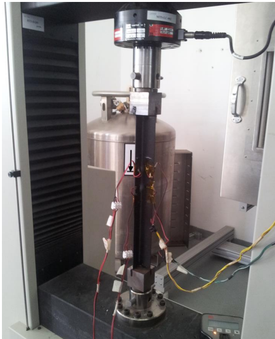
Figure 4: buckling test set-up for the stringer
