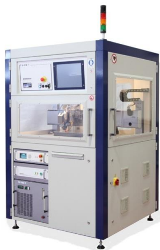
Figure 3: view of the induction welding machine (on the left) and detail of the welding head (on the right)
