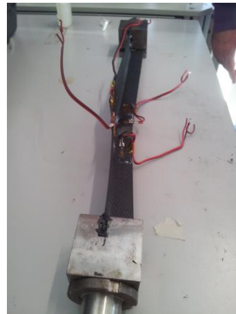
Figure 6: the stringer after the buckling test
