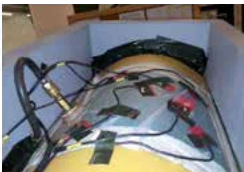
Anbringen der Temperaturfühler Placement of the temperature sensors
