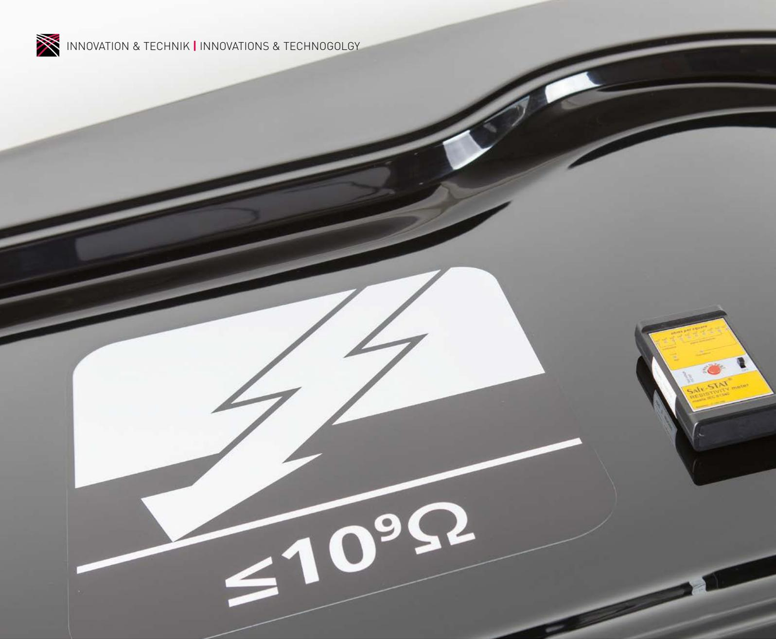
Dust-free surfaces thanks to the absence of electrostatic charging: The carbon-nanotubes in the new BÜFA®-Gelcoat convert non-conductive synthetics into electrically conductive materials. (photo BÜFA)
