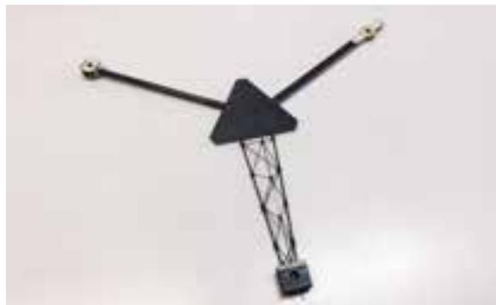
Three carbon-based arm constructions: the team opted for the fine lattice-frame construction (below).
