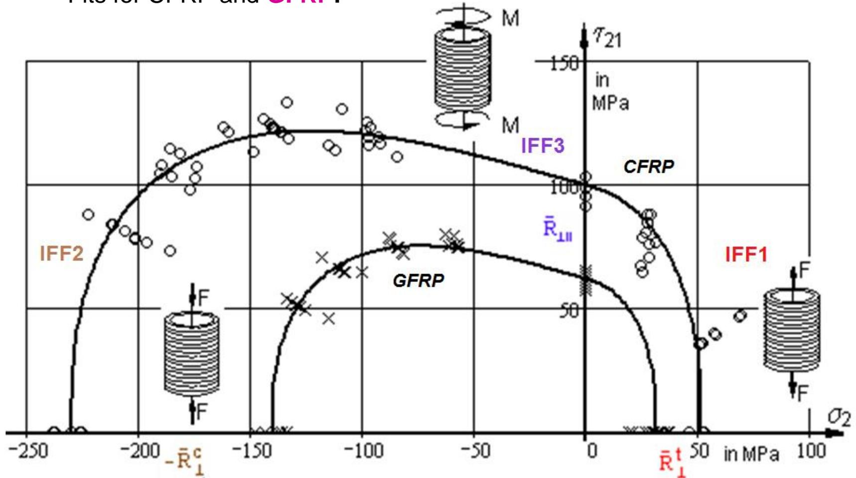
$$Eff = \left( \frac{\sigma_2^t}{\bar{R}_2^t} \right)^m + \left( \frac{-\sigma_2^c}{\bar{R}_2^c} \right)^m + \left( \frac{|\tau_{12}|}{\bar{R}_{\perp\parallel} - \mu_{\perp\parallel} \cdot \sigma_2^c} \right)^m = 1$$
