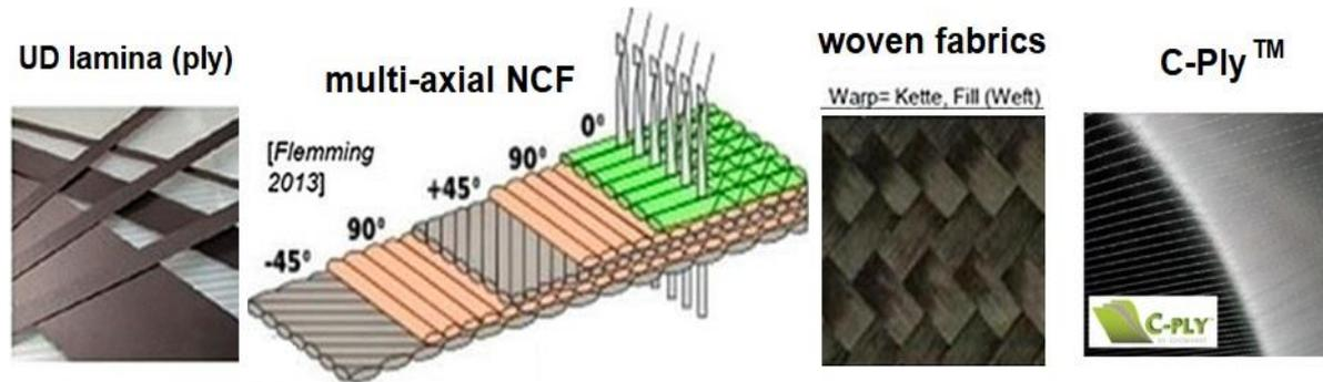
Fig.2, Visualization of applicable closed fiber reinforcing semi-finished products:(left) UD-layer (ply, lamella in CE), composing traditional laminates, stitched Non-Crimped Fabrics (NCF) and woven fabric, (right) novel deliverable C-ply™ = balanced angle ply (see [CUN §3])
