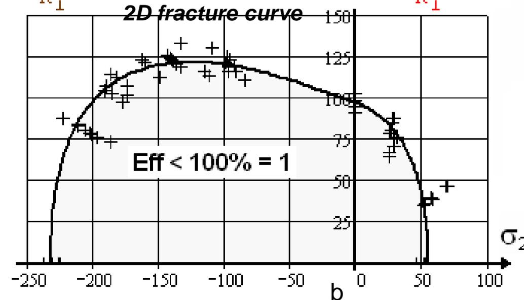
$$(Eff^{\perp\sigma})^m + (Eff^{\perp\tau})^m + (Eff^{\perp\parallel})^m = 1$$
