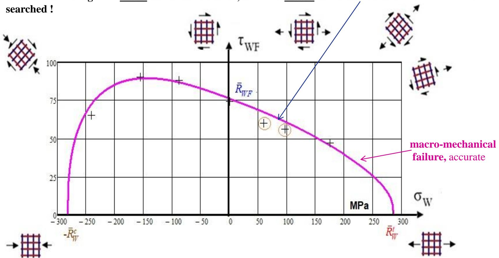
Off-axis coupon tests, Failure envelope . (data set Siemens AG).  $m = 2.6$
