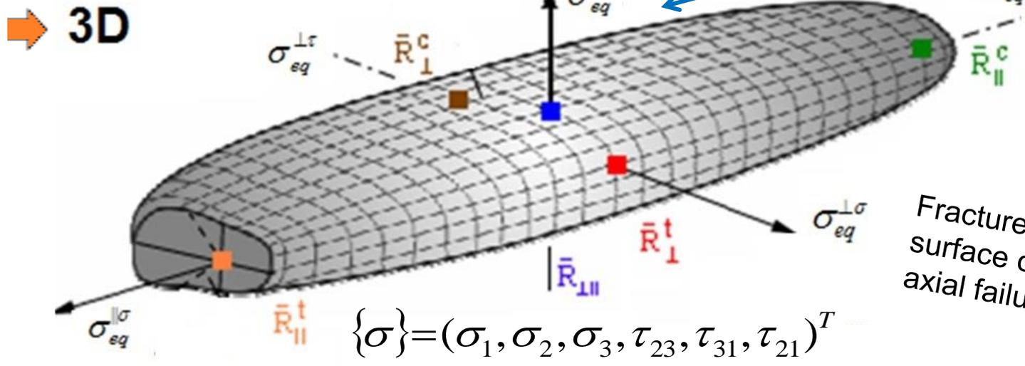
Fracture Body = smoothed surface of the ends of the multi-axial failure stress vectors
