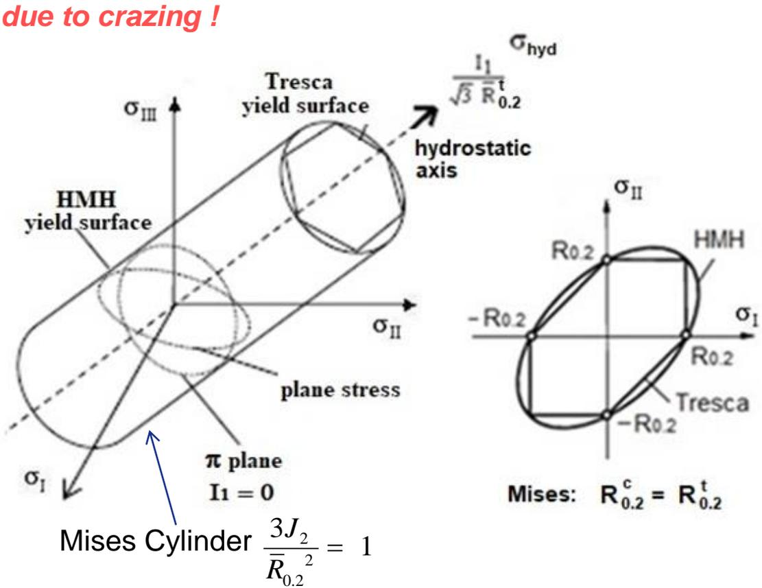
**Crazing failure** occurs which shows an increase in volume due to the formation of tension-elongated fibrils [CUN§4.1] and **shear yielding SY** does not.
