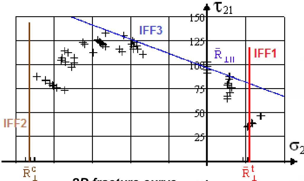
Mapping of course of IFF test data in a pure mode domain by the *single Mode Failure Conditions*.  $m = 2.7$
