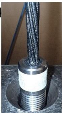
Fig.8-4: Carbon Fiber Composite Cable (CFCC) from Tokyo Rope, cable strand diameter 12.5 mm E-Modulus 155000 N/mm 2 , T_{max} = 130 °C. Static tensile tests: fracture load 274 kN per cable or strength 3000 N/mm 2 per cable strand (Kabellitze) [from presentation F. Jesse]
