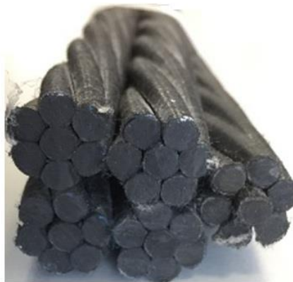
Fig.8-4: Carbon Fiber Composite Cable (CFCC) from Tokyo Rope, cable strand diameter 12.5 mm E-Modulus 155000 N/mm 2 , T_{max} = 130 °C. Static tensile tests: fracture load 274 kN per cable or strength 3000 N/mm 2 per cable strand (Kabellitze) [from presentation F. Jesse]
