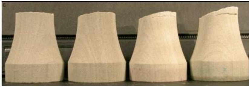
Fig.26-8, Sandstone: Fracture pictures of Berea sandstone from [Lan19].
