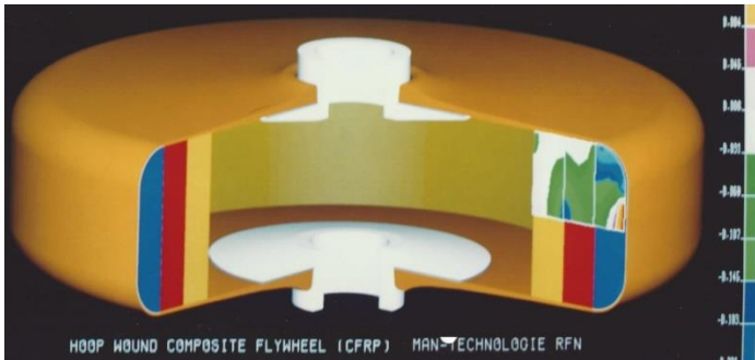
(left) FEA of a delamination-less energy storing fly wheel. (right) Development of a braided CFRP hip
