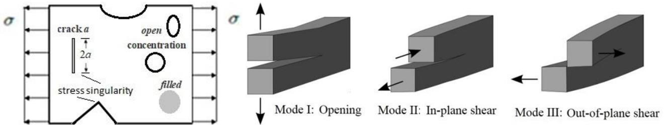
Fig. 4: (left) Stress concentrations and stress singularities under uni-axial stressing.
