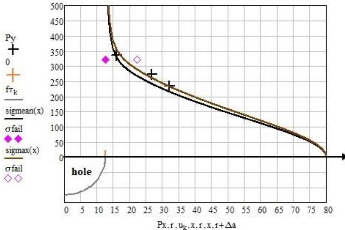
Fig.10: (a) Depiction of the FFM-based failure stress at ‘Onset-of-Cracking’ generating  $\Delta a$ .
