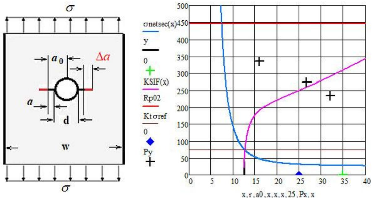
Fig.9: (left) Geometry of the fixed Open Hole Panel and its uniaxial loading.
