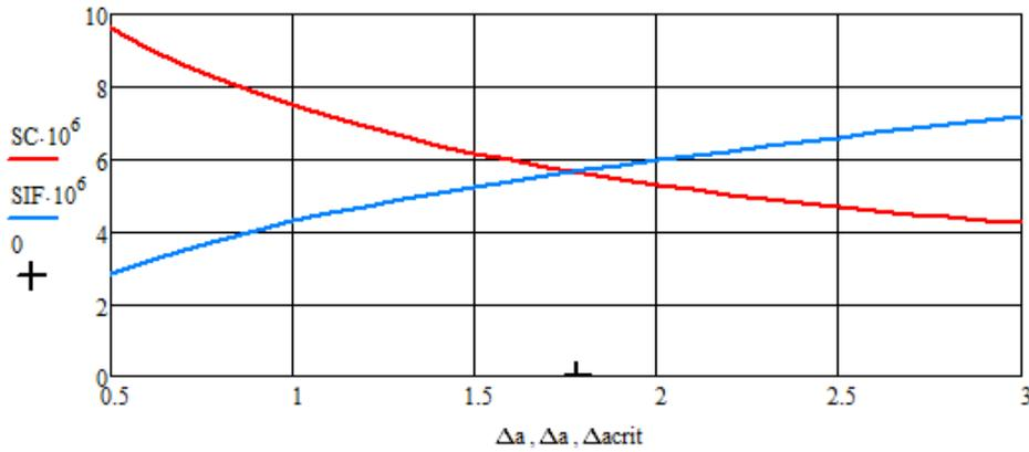
Fig.7,  $w = 36\text{mm}$ ,  $a_0 = 30\text{ mm}$ ,  $d = 6\text{ mm}$ : Representation of the course of the growing FM-portion (SIF) and the decaying Strength Mechanics portion (SC)
