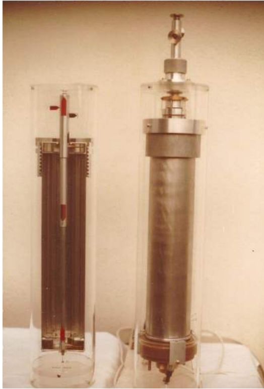
Dr. Zippe's Original Gas Ultracentrifuges for uranium-235 enrichment, single-stage . (secret), see [CUN25]
