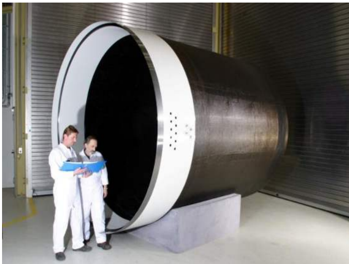
CFRP Booster section 2001
