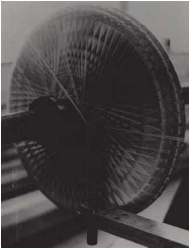
Fig.26-6: Pattern of a CFRP and of a AFRP fly wheel at MAN Technologie
