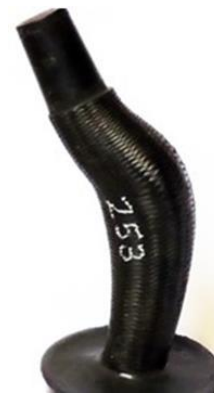
(left) FEA of a delamination-less energy storing fly wheel. (right) Development of a braided CFRP hip
